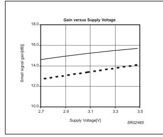
Figure 4. Gain vs. supply voltage
